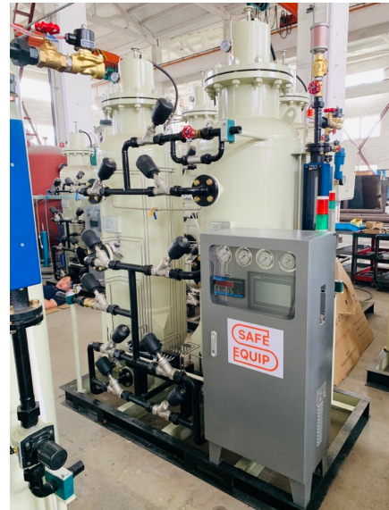
Valve train, instruments, and controls before shipment
