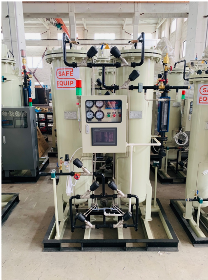
PSA equipment during factory assembly and inspection
