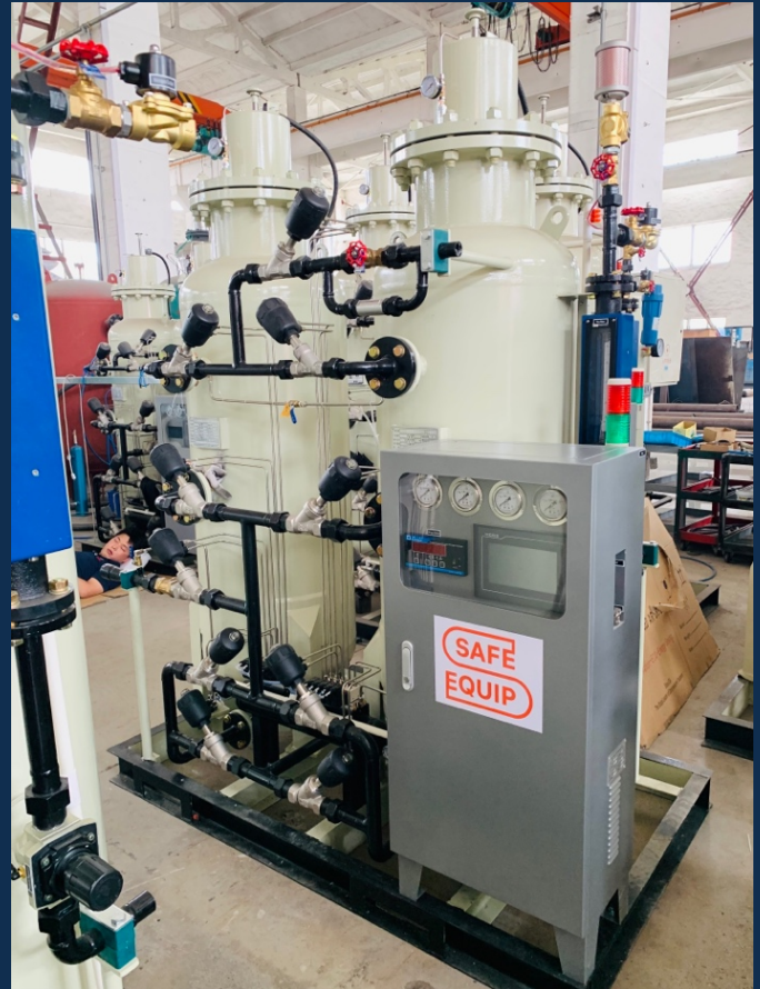
Safe Equip PSA equipment during factory assembly
